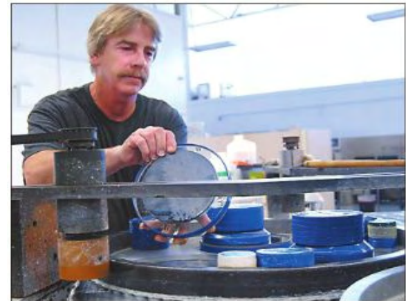
E.R. Precision's Scott Stevens removes a piece of silicon from the polisher.
